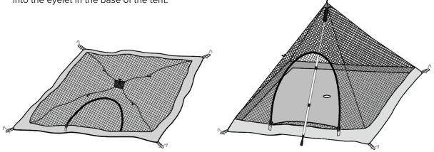
You may need to adjust the height of the pole depending on the hardness of the ground. It is always best not to extend the pole to the maximum initially, as you can adjust the height of the pole from the inside at any time.
